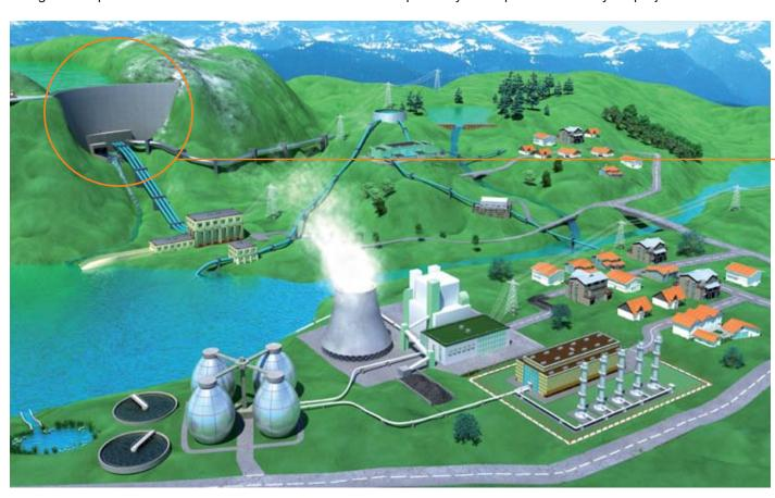
To prevent dams bursting or uncontrollably overflowing, almost all of today's dams are equipped with bottom outlets that are designed according to the dam's expansion capacity, which is determined by the reservoir's volume and its inflow and outflow. The bottom outlet is opened, closed and controlled by valves, frequently produced by VAG.
