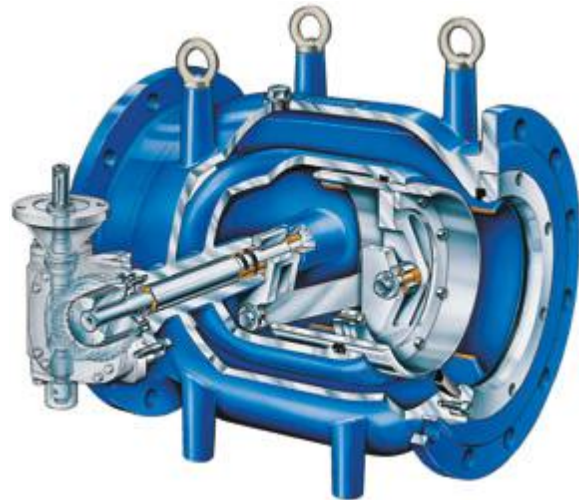
Figure 5: Sectional view of a VAG RIKO® Plunger Valve
